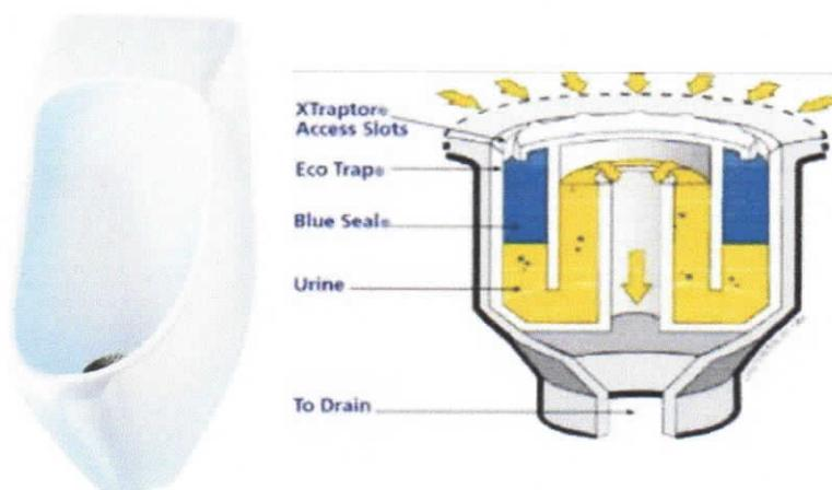
d. Approximately 1500 sanitary uses are possible with just 3 ounces of Blue Seal. When the Blue Seal liquid is gone, it is simply replenished. This only takes about 20 seconds to perform and the Eco Trap is not touched.
